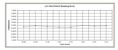
Installation Instructions: The LC is a single coil CT using a ferrite core. The core faces, when the top is lifted, must be clean of any dirt for the CT to stay within calibration. Due to the "corner affect" of a single coil CT, the conductor passing through the center should be centered and perpendicular to the CT window. You can secure the CT to the center conductor using nylon ties through the window and around the center conductor.
