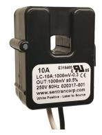
The LC45 Miniature Current Transformer is an indoor AC voltage output transducer designed for installation within breaker panels and industrial control cabinets. The snap top simplifies installation over wire sizes up to 0.4" diameter. The CT is provided with an internal resistor for an AC voltage output signal. Current ratio models are available depending on output current required, but the current ratio is limited due to coil winding space.
