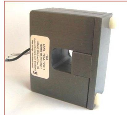
The Model 4AN4 Split Current Transformer is a low AC voltage output transformer designed to simplify the installation over insulated conductors. The transformer core material is extra thick nickel core for ultra precision measurement of AC current. Two screws are used to secure the top after closing. Standard turns ratio is 1250:1, but other ratios can be provided or we can set an output voltage using an internal.
